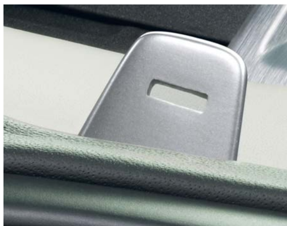
NEW - Gearshift Paddles - Aluminium Gearshift Paddles offered in high grade aluminium which is machine polished, anodised and hand brushed to provide exceptional wear resistance with a premium finish. Billet machined from solid aluminium. VPLVS0187MMU
